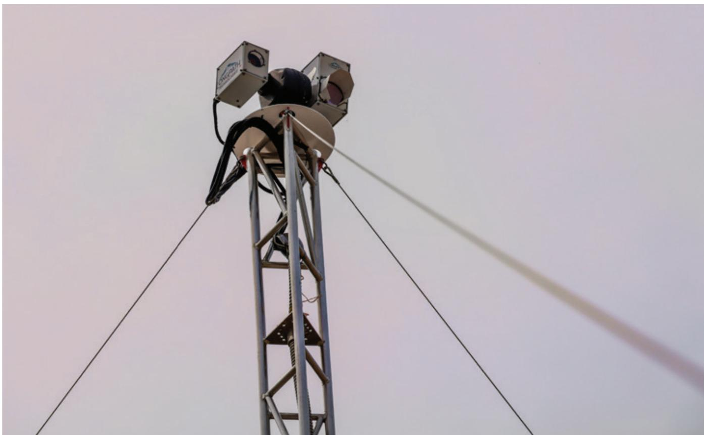
Figure 7: A close-up shot of LongPath's Continuous Open-Path Sensor, which utilizes invisible, eye-safe long-range lasers to detect methane-specific greenhouse gas molecules up to a 2.5-mile radius from installation.
