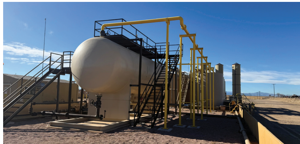
Figure 6: A surge vessel on a Bayswater location in the DJ Basin.
